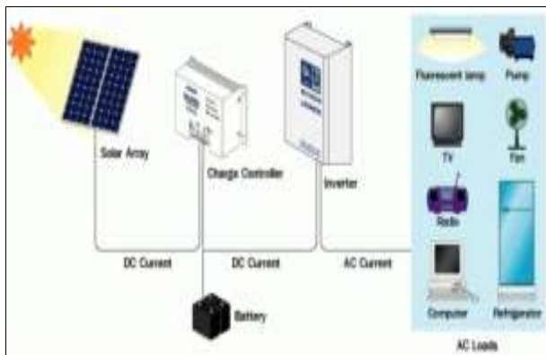
Gambar 2. Solar Home System
